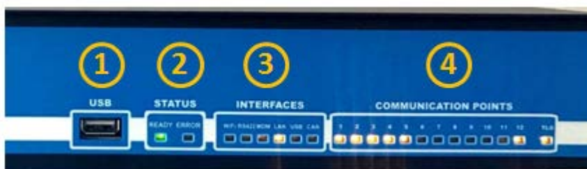
Figure 1 – FDC (Front Panel) – Indicators and connectors
