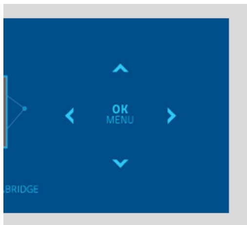
Figure 8 – RoSyS V2L Bridge (Top View) – Control keys position
