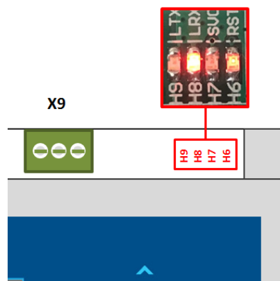
Figure 7 – RoSyS V2L Bridge – X9-related LEDs position
